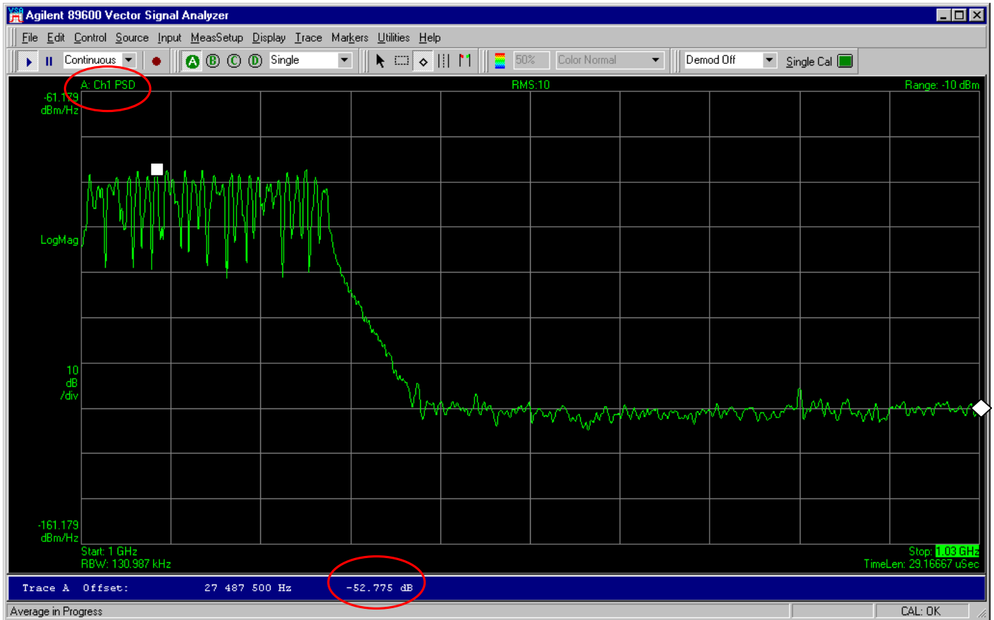
Figure 23: 89640A VSA Power Spectral Density Measurement of Signal Studio-802.11a Signal
